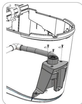
9. Tighten the three screws
